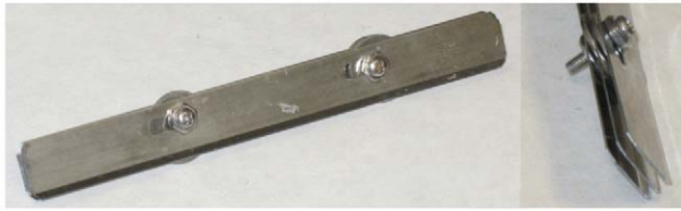
Figure 2. Multi-section scoring device, consisting of histology blades connected together, used to score the tissue embedded in agarose gel. Individual tissue slices are then made using a single histology blade.
