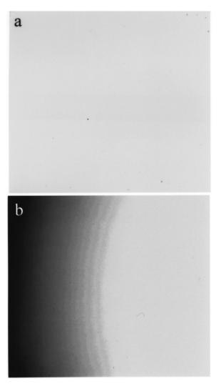
**Fig. 5** Light distribution on the 99% diffuse reflectance standard at view angles of (a) 0 and (b) 35 deg. Image contrast was adjusted to enhance visualization of the light distribution.
