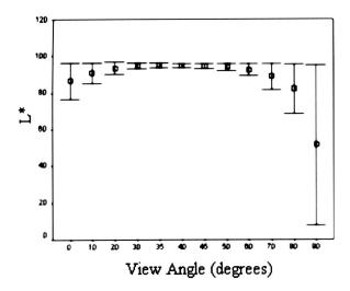
**Fig. 6** Example illustrating the dependence of  $L^*$  values on view angle. In this measurement, patches 2 to 21 comprised the ROI, and the optimal view angle was determined to be 40 deg (CV=1.2%).
