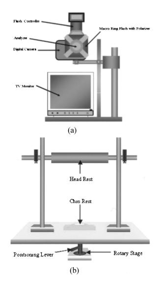
**Fig. 1** (a) Diagram of the cross-polarized diffuse reflectance imaging system and (b) of the head positioning device used to standardize images obtained from each subject.
