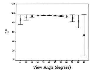
**Fig. 7** Effect of view angle on  $L^*$  in the white patch ROI corresponding to the PWS-simulating red patches on the mannequin head model. The white patches numbers corresponding to the red patches were 2 to 9, 11 to 12, 14 to 16, 19 to 20, 23 to 24, and 27. The optimal view angle was 35 deg with a CV of 0.4% ( $\mu$ , 95.87 and  $\sigma$ ,  $\pm$ 0.4).
