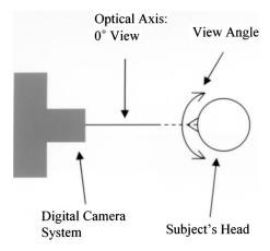
**Fig. 2** Schematic diagram for facial image acquisition. View angles, defined as the angle between the optical axis of the imaging system and medial facial plane, were selected by adjusting the rotation of the head-positioning device.
